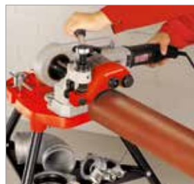
Use with roll grooving tool ROGROOVER
