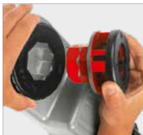
Easy insertion of the die heads
