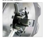
Automatic die heads with quick adjustment of thread size, automatic thread length and finely adjustable thread depth without recentering
