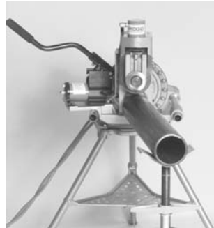
Figure 12 – Offset Pipe on 918 in FORWARD Position
