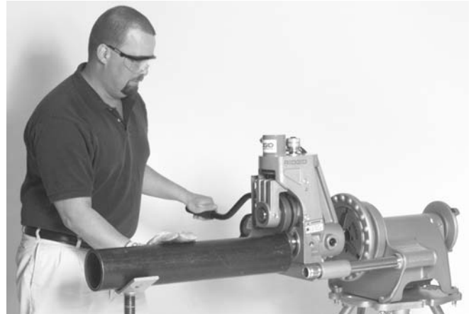
Figure 15 – Applying Pressure on Pipe with Power Drive in FORWARD Mode
