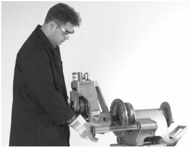
Figure 2 – Installing on 300 Power Drive
