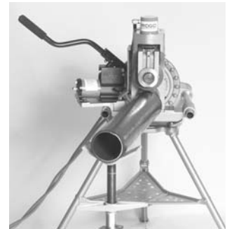
Figure 13 – Offset Pipe on 918 in REVERSE Position
