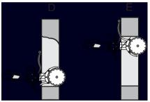
The blade guards are designed to easily adapt to how deep in the work piece the power cutter is moved.
