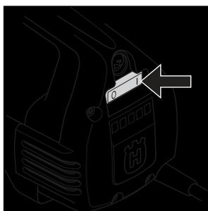
The power switch should be used to start and stop the machine.
