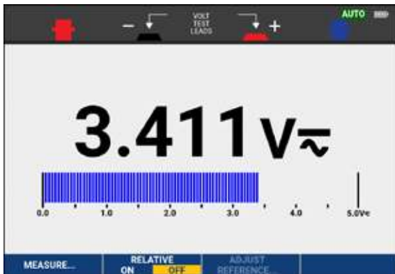
The built-in multimeter provides convenient precision measurements
