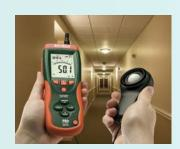
Extech's HD450 measures light level up to 40 kFc (400 kLux) with a 0.01 Fc (0.1 Lux) resolution. Features: Peak mode (10µs), Relative mode, Min/Max, Data Hold, backlit LCD display with 40-segment bargraph, and a rugged double molded housing. In addition, the datalogger function can automatically store up to 16,000 readings or manually store/recall up to 99 readings.
