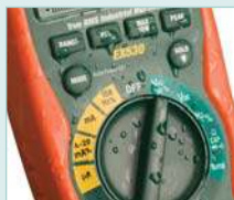
Double molded for rugged, waterproof (IP67) protection
